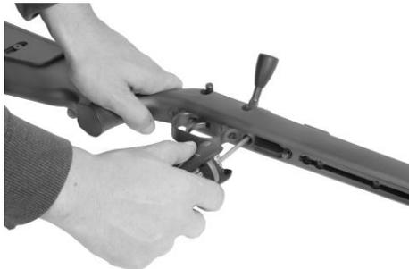
Open the screw on the UIT-rail that holds the action in the stock and take it out. An Allen key size 3 mm is required to unscrew the two action screws.
