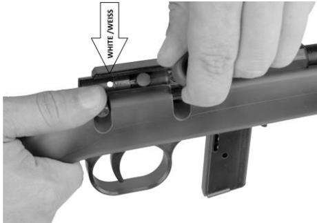
Lift the safety lever in the upper position in order to disengage the safety. When the safety is disengaged, a red dot is visible.
