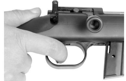
The rifle is fitted with a two stage trigger. Press the trigger gently until the first stage of the trigger. The rifle will fire by further increasing the pressure. Make sure always to point the rifle into a safe direction.
