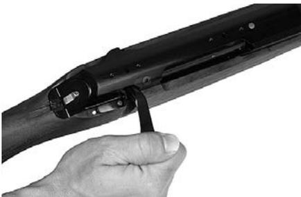
**Note that the guidance slot of the bolt sleeve and the bolt body line up.**
