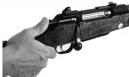
With the thumb in the indentation of the tensioner, press forwards hard until it engages. Releasing the safety exposes a red spot on the housing.
