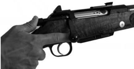
From the compressed position the rifle can be decocked by pressing and gently releasing the cocking handle.
