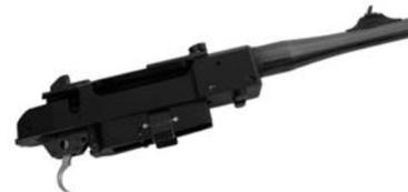
Push the Barrel (1) from the front into the Action (2). Ensure that the sight or the index groove is uppermost, or the inscription (serial No.) is on the right. The fine tolerances require the barrel to be aligned exactly with the housing. When the barrel is fully inserted, use a 5 mm socket key to tighten the clamp screws (3 and 4) hand tight.
