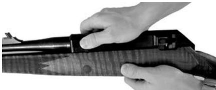
Put the action with barrel (muzzle forwards) in the stock. First insert the trigger, and tilt the action into the stock. This should require no force. With the action in the stock, hand tighten the action locating screws with a socket key (5 mm). The screws should not project beyond the trigger guard plate.
