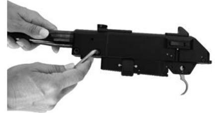
the socket-head screws on the side of the housing. When the screws are loose the barrel can be withdrawn from the housing.
