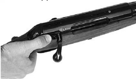
The standard safety is a trigger safety, which operates on the sear. When the safety catch is in the rear position, the gun is safe and the breech cannot be opened (chamber lock active if this option was chosen at purchase time). When the safety is in the forward position (red spot visible), then the gun is not safe, and the breech can be opened.
