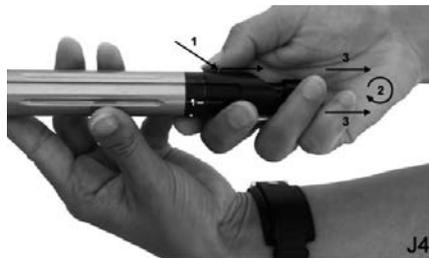
Reassembling has to be done in the opposite direction. Introduce the firing pin into the bolt body.
