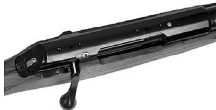
The mounting surface as well as the threaded holes and the two plain locating holes offers many possibilities for your own scope mount.
