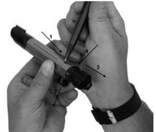
Now the bolt head can be removed forwards without any problems (3). A new bolt head can be put on the same way. Ensure that both flat areas fit together (4). Fix the bolt assembly by inserting the cross bolt.
