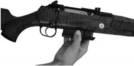
On pressing the magazine latch from both sides simultaneously the magazine will fall out.
