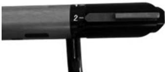
Moving the pin on the upper side of the bolt sleeve backwards and turning it clockwise in position 1 at the same time the cocking piece will be opened. Now it can be removed backwards.
