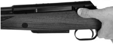
Free the bolt by turning the bolt handle through 60°, pull it to the rear while pressing the bolt stop release on the left (in any case, before the bolt is in its rearmost position). The bolt can now be easily removed from the housing. To replace the bolt in the housing, ensure it is centred and introduce it with a slight turn to the right.
