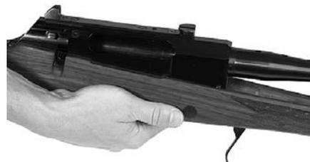
Put the action with barrel (muzzle forwards) in the stock. First insert the trigger, and tilt the action into the stock. This should require no force.
