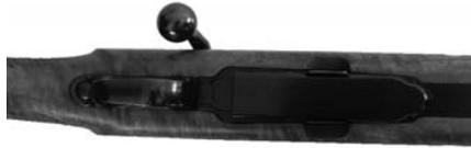
Remove the magazine for safety reasons and ensure that the chamber is clear of ammunition. Remove the bolt.
